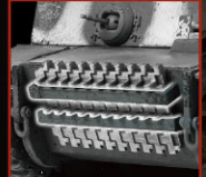
TRACK LINK RACK Spare track link rack holds the spare track with the upper and lower beam.
